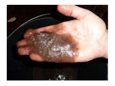
In colder climates, paraffinic components in MGO can begin to crystallize into large wax structures. This can occur even before reaching freezing temperatures, as some fuels may begin to solidify well above 0°C. These crystals can obstruct filters, fuel lines and injectors, creating severe operational and safety risks. In extreme cases, fuel may become unpumpable, resulting in potential propulsion loss.
